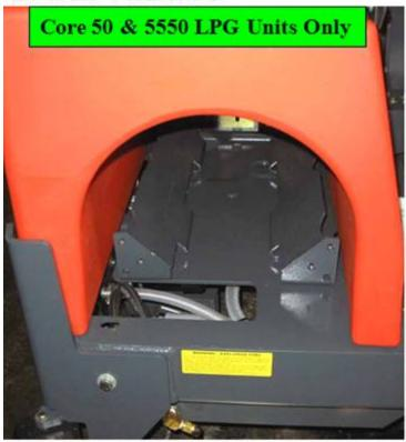
Close valve on LP tank. Disconnect LP tank hose from LP tank and remove LP tank from unit.
